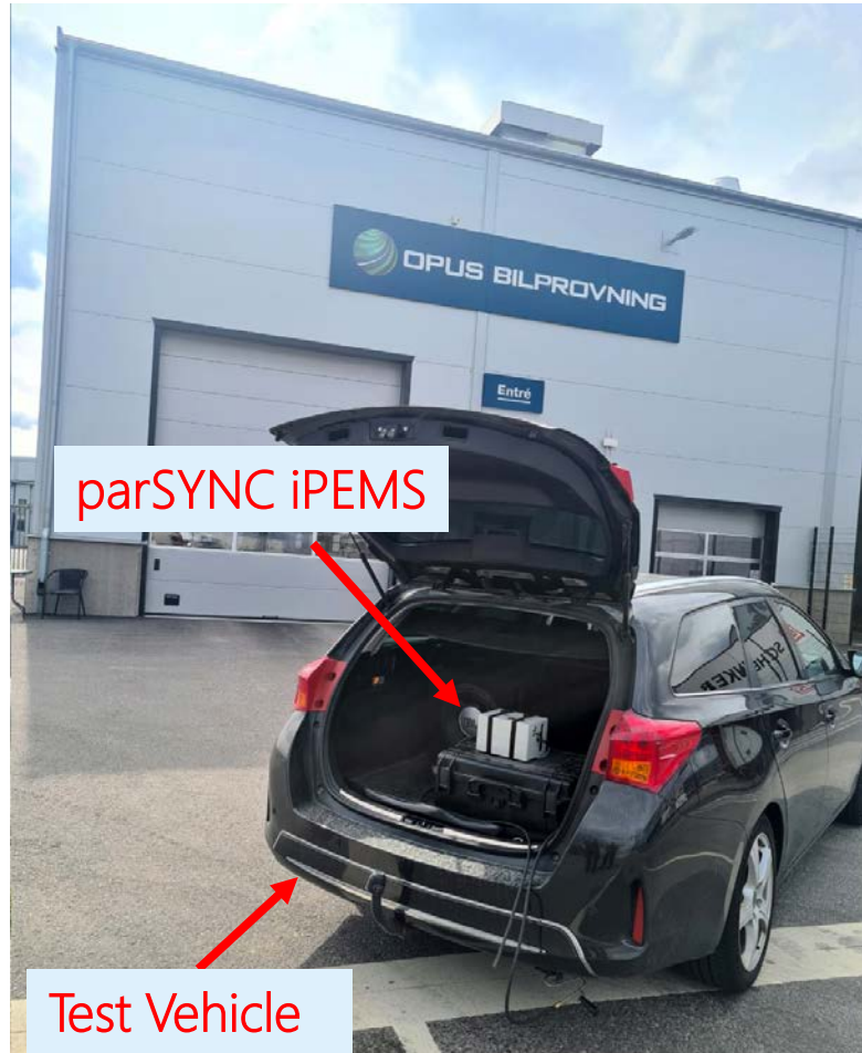
parSYNC warmup and zeroing while vehicle is being prepared
